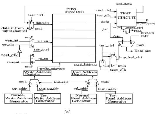
**Fig-1:-** Hardware implementation of the test process for the FIFO buffers
